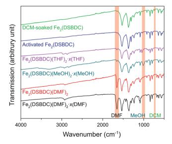
Fig. 2 IR spectra of various forms of  $Fe_2$ (DSBDC). Characteristic peaks of DMF, MeOH, and DCM are highlighted.
