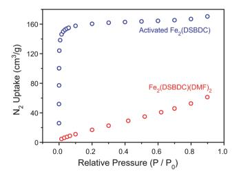
Fig. 4  $N_2$  sorption isotherms of Fe<sub>2</sub>(DSBDC)(DMF)<sub>2</sub> and activated Fe<sub>2</sub>(DSBDC).
