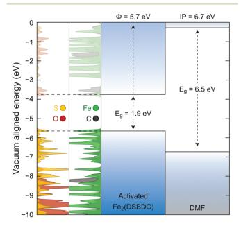
Fig. 6 Electronic band structure of activated Fe<sub>2</sub>(DSBDC) and molecular orbital energy levels of DMF. The left two panels are projected density of states in  $Fe_2(DSBDC)$ .  $E_g$  represents the band gap for Fe<sub>2</sub>(DSBDC) and the HOMO-LUMO gap for DMF.  $\Phi$  and IP represent work function and ionization potential, respectively.
