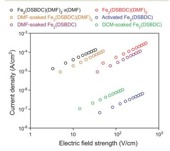
Fig. 5 Plots of current density *versus* electric field strength of various forms of Fe<sub>2</sub>(DSBDC).
