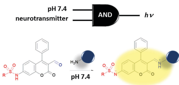
Fig. 14 AND logic gate for potential detection of exocytosed amine-bearing neurotransmitters.
