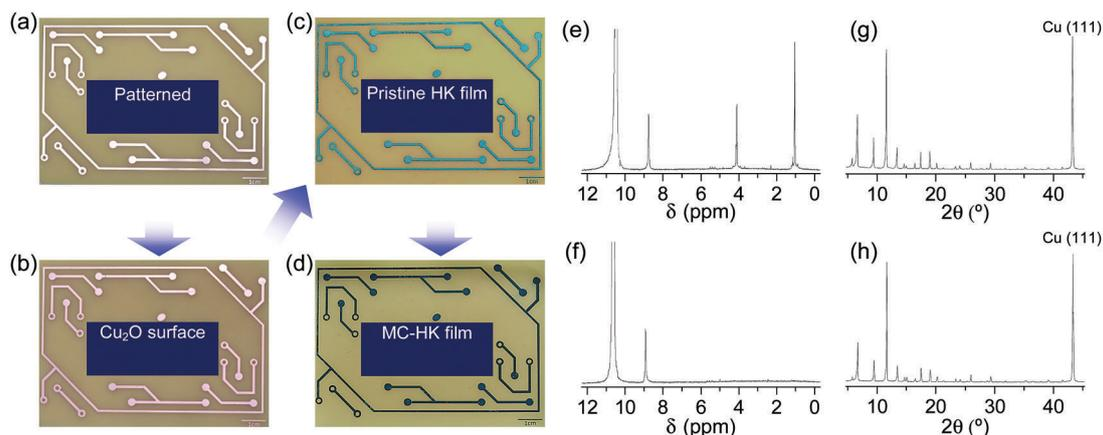
Fig. 16 Photographs of the (a) patterned Cu substrate, (b) surface-oxidized Cu substrate (Cu<sub>2</sub>O/Cu), (c) pristine-HK film synthesized on the Cu substrate, and (d) DCM-treated pristine-HK film. (e and f) <sup>1</sup>H NMR spectra and (g and h) XRD patterns of pristine-HK films (e and g) before and (f and h) after DCM treatment. Reprinted (adapted) with permission from ref. 68. Copyright (2015) American Chemical Society.
