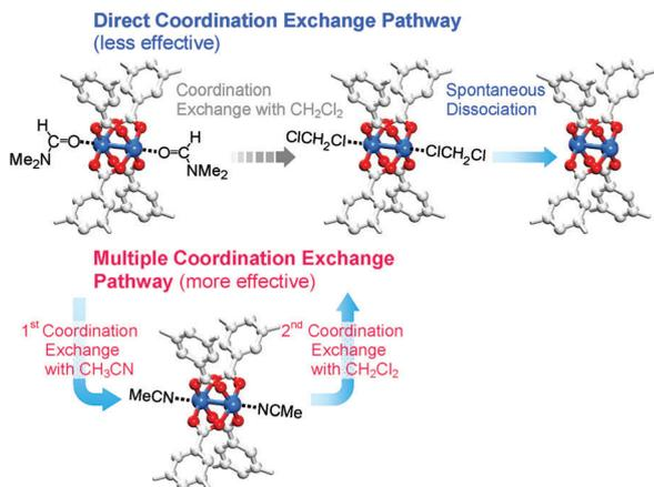
Fig. 8 Schematics illustrating direct and multiple coordination exchange pathways for the activation of the paddle wheel-like ( $\text{Cu}^{\text{II}}\text{)}_2$  node of HKUST-1. Hydrogen atoms bound to the carbon atoms in the benzene moieties are omitted for clarity. Reprinted (adapted) with permission from ref. 69. Copyright (2017) American Chemical Society.
