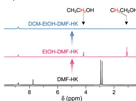
Fig. 9  $^1\text{H}$  NMR spectra of DMF-coordinated HKUST-1 before and after initial solvent treatment with (a) MeCN, (b) MeOH, and (c) EtOH and after subsequent solvent treatment with DCM. NMR spectra were measured after the powder samples were completely dissolved in  $\text{D}_2\text{SO}_4$ . Reprinted (adapted) with permission from ref. 69. Copyright (2017) American Chemical Society.
