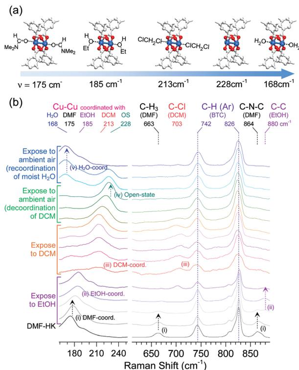
**Fig. 11** (a) Illustrations of DMF-coordinated, EtOH-coordinated, DCM-coordinated, open-state, and  $\text{H}_2\text{O}$ -coordinated ( $\text{Cu}^{\text{II}}_2$ ) centers in HKUST-1 (from left to right). (b) Successive changes of the *in situ* Raman spectra of DMF-coordinated HKUST-1 during sequential exposure to EtOH, DCM, and ambient air. Reprinted (adapted) with permission from ref. 69. Copyright (2017) American Chemical Society.
