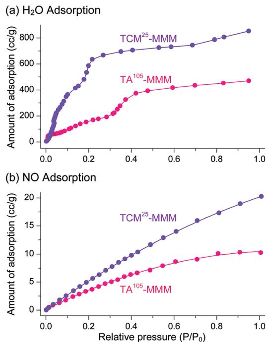
**Fig. 20** (a)  $\text{H}_2\text{O}$  and (b)  $\text{NO}$  adsorption isotherms of  $\text{TA}^{105}$ -MMM and  $\text{TCM}^{25}$ -MMM. The isotherms for the  $\text{TCM}^{25}$ -MMM sample were measured after applying vacuum at room temperature for 4 h. Reprinted (adapted) with permission from ref. 70. Copyright (2018) American Chemical Society.
