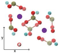
Fig. 3 Representation of a single unit cell of HA (Ca<sub>10</sub>(PO<sub>4</sub>)<sub>6</sub>(OH)<sub>2</sub>) projected on the xy plane. Each purple circle represents two aligned Ca1. Colour key Ca1: purple, Ca2: light blue, P: green, O: red, H: white.
