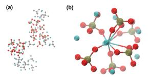
Fig. 8 Solution II: (a) aggregates after 5 ns; (b) detail of one of the Posner-like clusters formed with formula  $Ca_9(PO_4)_6$ . Colour key Ca: light blue, P: green, O: red, atoms not forming Posner's clusters: grey.
