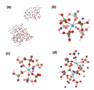
Fig. 6 Solution Ia: (a) aggregates after 5 ns; Posner-like clusters with chemical formulas (b)  $[Ca_3Na_4(H_2PO_4)_3(HPO_4)_3]^+$  and (c)  $[CaNa_6(HPO_4)_6]^{4-}$ . (d) Two Posner-like clusters sharing three phosphate groups, formula [Ca<sub>6</sub>Na<sub>8</sub>(H<sub>2</sub>PO<sub>4</sub>)<sub>4</sub>(HPO<sub>4</sub>)<sub>5</sub>]<sup>6+</sup>. Colour key Ca: light blue, Na: dark blue, P: green, O: red, atoms not forming Posner's clusters: grey.
