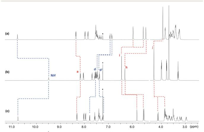
Fig. 2 Comparison of the partial <sup>1</sup>H NMR spectra (500 MHz, CDCl<sub>3</sub>) of (a) suit[1]ane 6a, (b) an equimolar solution of 1 and 7 and (c) suit[1]ane 6b (\* =  $CHCl_3$ ). Labelling scheme is shown in Scheme 2 for 1 and 7.
