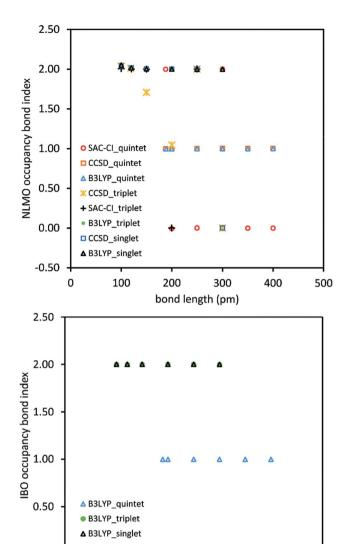
Fig. 1 For stretched bonds, the bond order does not resemble the occupancy bond index. The NLMO and IBO occupancy bond indices for stretched  ${\rm O_2}$  are shown in the top and lower graphs, respectively. The bond order should smoothly decrease towards zero as the bond length increases, but the occupancy bond indices do not produce this trend.
