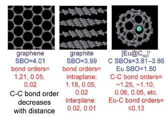
Fig. 10 DDEC6 bonding analysis for three nanostructured materials with a high content of aromatic carbon atoms: graphene, graphite, and  $[{\rm Eu@C_{60}}]^+$ .
