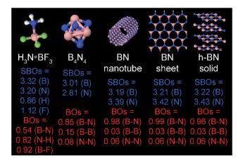
Fig. 11 DDEC6 bonding analysis for five structures containing B-N bonds:  $H_3N \cdot BF_3$ ,  $B_4N_4$  molecule, BN nanotube, BN sheet, and h-BN solid.
