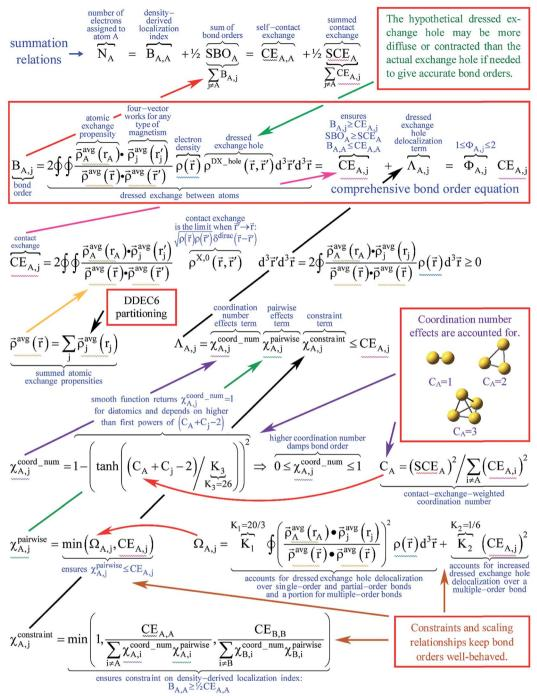
Fig. 3 Diagram showing key relationships between equations for computing DDEC6 bond orders. Red boxes enclose the main equation and high level concepts. Arrows indicate the sources of selected inputs or concepts used in each equation. Each variable reappearing in several different equations is marked with a specific color of squiggly underline (note: sometimes a variable reappears inside a summation). Blue text annotations explain key terms.
