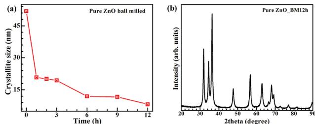
Fig. 2 (a) Crystallite size reduction as a function of milling time. After 10 h, the reduction in size is minimal. Hence, we have restricted the milling time to 12 h. (b) XRD of ball milled zinc oxide powders after 12 h. The particles are crystalline with peak broadening due to size reduction. The crystallite size is calculated from the XRD pattern using Debye–Scherrer formula.
