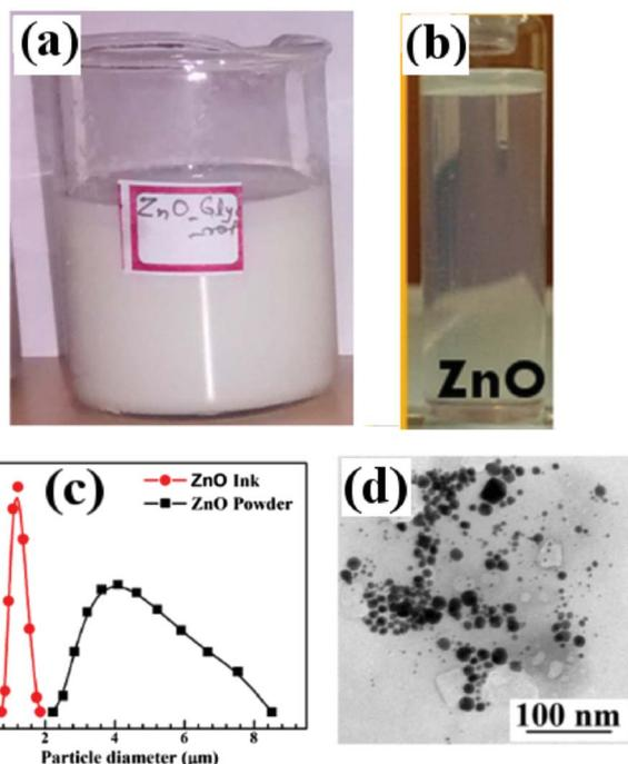
**Fig. 4** Picture of the (a) as-prepared unfiltered and, (b) filtered glycerol (PZ1) ink. (c) Particle size distribution of as received ZnO powder and after ball milling for 12 h. The as prepared ink is filtered using a 200 nm pore size filter, since the print head in the commercial inkjet printer was 25 µm and the particle size cannot be larger than 250 nm (100 times smaller). (d) TEM of the filtered ink shows that most of the particles have size smaller than 100 nm.
