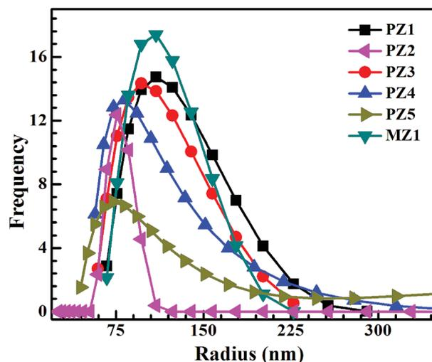
Fig. 3 Comparison of the particle size distribution as a function of solvent and ZnO loading. PZ1 and PZ3 correspond to glycerol and ethylene glycol inks respectively and show similar size distribution. PZ5 is ethylene glycol ink with double the ZnO loading. The particle size distribution for PZ5 is wider with a longer tail due to this higher particle loading.
