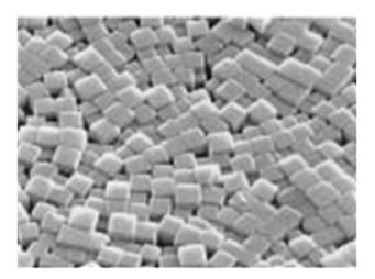
Fig. 2 Typical morphology of LTA zeolite crystal monolayer (magnification ×1200). Reprinted with permission from A. Kulak, Y. J. Lee, Y. S. Park and K. B. Yoon, Orientation-Controlled Monolayer Assembly of Zeolite Crystals on Glass and Mica by Covalent Linkage of Surface-Bound Epoxide and Amine Groups, *Angew. Chem.*, 2000, **112**, 980–983. Copyright (2000) John Wiley and Sons.<sup>72</sup>
