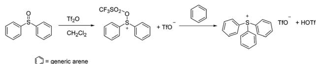
Scheme 1 Common synthesis of triarylsulfonium triflate salts.
