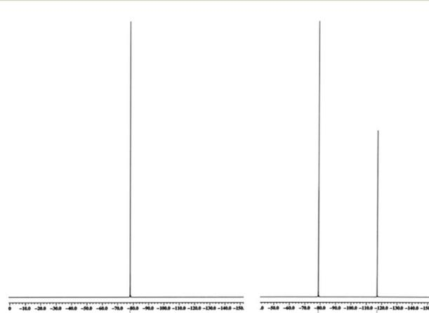
Fig. 2 <sup>19</sup>F-NMR of Ph<sub>3</sub>S<sup>+</sup> TfO<sup>-</sup> (left) with its single resonance from CF<sub>3</sub>, and after anion exchange to form the corresponding BETI salt with both CF<sub>2</sub> and CF<sub>3</sub> resonances.
