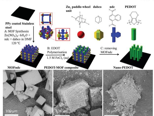
Fig. 1 Schematic diagrams illustrate the experimental steps in sequence: synthesis of MOFndc on PPy coated stainless steel, chemical polymerisation of EDOT in MOFndc, and formation of nano-PEDOT after removing PEDOT. SEM images obtained with back-scattered electrons (BSE) reveal the morphologies of the products at the steps A–C. 3D schematics are created with open sourced software available from http://www.openscad.org/.
