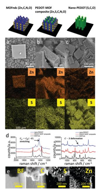
Fig. 2 BSE-SEM images with EDS mappings of Zn and S for (a) MOFndc, (b) PEDOT-MOF composite and (c) nano-PEDOT. Raman spectra (d) extended scan (left) and static scan (right) around 700 cm<sup>-1</sup> Raman shift. (e) Energy filtered transmission electron microscopy (EFTEM) images with EELS mappings of C (K-edge, 284 eV), S (L-edge, 165 eV) and Zn (L-edge, 1020 eV).
