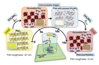
Fig. 7 Methylamine gas induced perovskite formation. Illustration of the setup used for processing perovskite at room temperature from simple precursors of  $CH_3NH_2$  gas; the  $Pbl_2$  film is depicted in the lower middle part of the figure. Reproduced from ref. 77 with permission from The Royal Society of Chemistry.
