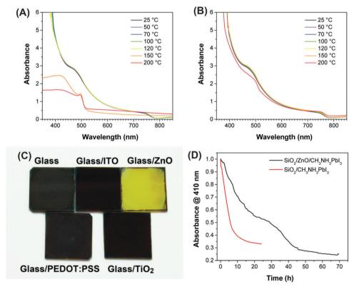
Fig. 15 Absorbance spectra of MAPbl $_3$  films deposited on different substrates. (A) ITO/ZnO or (B) ITO substrates and annealed at various temperatures for 5 min. (C) Photograph of MAPbl $_3$  films on various substrates after heating to 100 °C for 20 min. (D) Normalized absorbance at 410 nm as a function of time for SiO $_2$ /ZnO/MAPbl $_3$  and SiO $_2$ /MAPbl $_3$  films exposed to 98  $\pm$  2% R.H. Reproduced from ref. 124, Copyright 2015 American Chemical Society.
