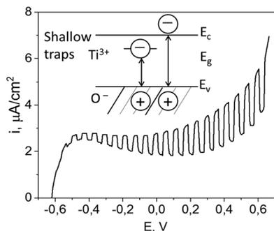
Fig. 4 Photochemical behavior of  $\text{TiO}_2$ .  $I$ - $V$  curve of blank  $\text{TiO}_2$  with chopped illumination. Inside schematic shows zone diagram of  $\text{TiO}_2$  and suggests possible trapping in forbidden zone that may explain photo-activity during irradiation at 405 nm.
