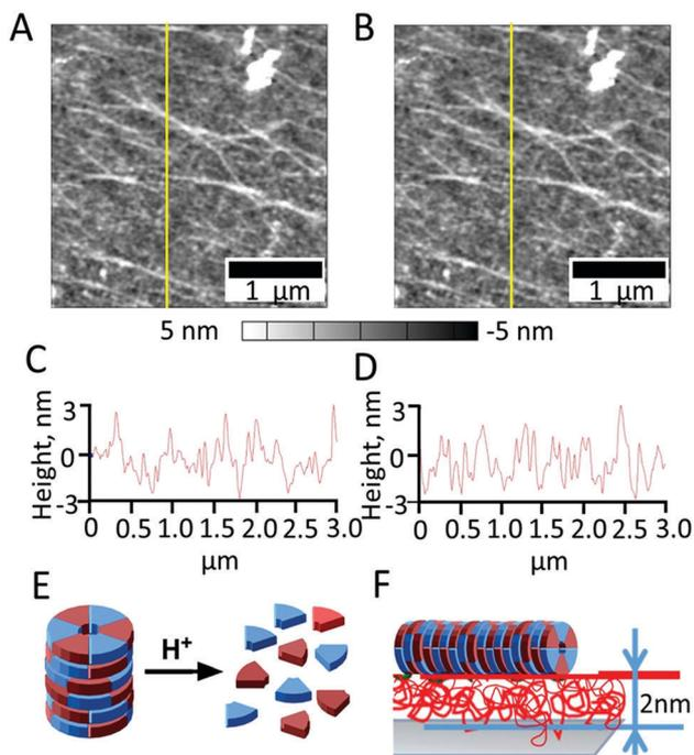
**Fig. 9** AFM images of Layer-by-Layer (LbL) deposited chitosan films on titania followed by TAP/CyCo6 deposition before (A) and after 10 min of irradiation with 9 mW intensity from a 405 nm laser (B), with the corresponding cross sections (C and D). Schematics showing TAP-CyCo6 disassembly resulting from pH-change, and (E) chitosan nanolayer as a proton sponge that affectively protects TAP-CyCo6 supramolecular polymers from disassembly (F).
