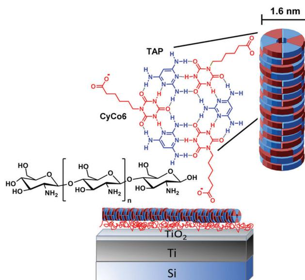
Fig. 1 Light sensitive TiO<sub>2</sub> layer on Si/Ti (negatively charged), positively charged layer of chitosan and negatively charged rosette-based supramolecular polymers of coassembled triaminopyrimidine (TAP) and cyanuric acid modified with hexanoic acid (CyCo6).
