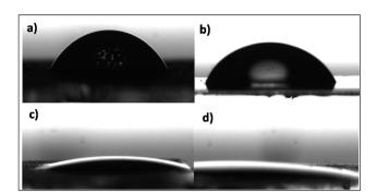
Fig. 4 Contact angle measurements of (a) ITO (b) APTES/nZrO $_2$ /ITO (c) serine/nZrO $_2$ /ITO and (d) anti-CYFRA-21-1/serine/nZrO $_2$ /ITO electrodes.
