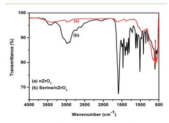
Fig. 2 FTIR spectra of (a)  $nZrO_2$  nanoparticles and (b) serine functionalized  $nZrO_2$  nanoparticles (serine/ $nZrO_2$ ).
