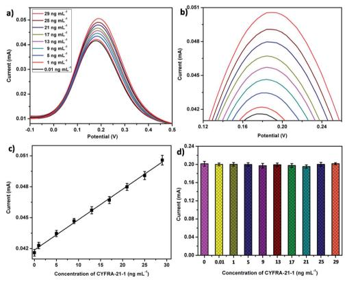
Fig. 5 (a) DPV response studies of BSA/anti-CYFRA-21-1/serine/nZrO<sub>2</sub>/ITO immunoelectrode as a function of CYFRA-21-1 concentration  $(0.01-29 \text{ ng mL}^{-1})$ , (b) magnified view of peak current response, (c) calibration curve between the magnitude of peak current and concentration of CYFRA-21-1 (ng mL<sup>-1</sup>) and (d) A control experiment of serine/nZrO2/ITO electrode as a function of CYFRA-21-1 concentration  $(0.01-29 \text{ ng mL}^{-1})$ .
