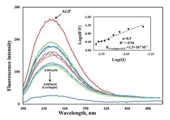
Fig. 2 Fluorescence emission spectra were measured for AGP along with corilagin in 0.1 M phosphate buffer with pH 7.2,  $\lambda_{\rm ex}=285$  nm, and temperature = 25  $\pm$  1 °C. Free AGP (0.001 mM) and free AGP with different concentrations of corilagin, 0.001–0.009 mM. Insert: plot of log(dF/F) against log[Q].  $\lambda_{\rm ex}=285$  nm and  $\lambda_{\rm em}=340$  nm.
