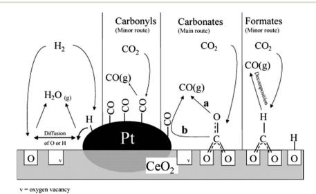
Fig. 7 Proposed rWGS mechanism on the Pt/CeO<sub>2</sub> interface. Reproduced with permission from the American Chemical Society (from ref. 109).
