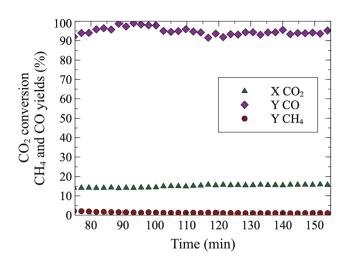
Fig. 3 Reverse water gas shift reaction over 78.3 mg of  $La_{0.75}Sr_{0.25}$ - $FeO_3$  at 550 °C. Total flow 50 sccm (10%  $H_2$  10%  $CO_2$  v/v, He balance). Previously, catalyst was reduced for 20 min in 10%  $H_2$ /He at 550 °C.
