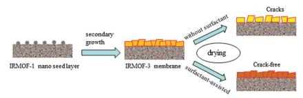
Fig. 11 Schematic representation of the fabrication of crack-free IRMOF-3 membranes using the surfactant-assisted drying method.
