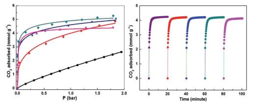
Fig. 9 (Left) CO<sub>2</sub> adsorption isotherms of MIL-101(Cr) before and after PEI loading at 25 °C. Symbol: ■ MIL-101, ● PEI-MIL-101-50, ★ PEI-MIL-101-75, ◆ PEI-MIL-101-100 and ▲ PEI-MIL-101-125. (Right) Cycling CO<sub>2</sub> adsorption kinetics of PEI-MIL-101-100. Reproduced from ref. 62 with permission of Nature Publishing Group.
