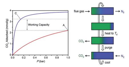
Fig. 10 (Left) CO<sub>2</sub> adsorption isotherms at 40 °C and 150 °C. Reprinted from ref. 59. Copyright 2012 American Chemical Society. (Right) Schematic representations of temperature swing adsorption. Reprinted from ref. 73 with permission from Royal Society of Chemistry.
