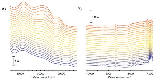
Fig. 5 Time evolution (from orange to blue) of the *operando* UV-vis-NIR DRS spectra of the fresh Cr/SiO<sub>2</sub> Phillips-type catalyst (CS sample) during the oligo-/polymerisation of ethylene, in the UV-vis (A) and the NIR (B) region.
