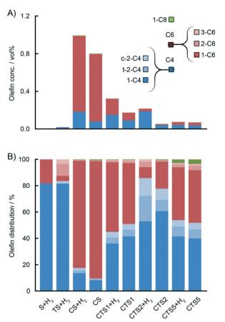
Fig. 7 GC analysis of the gas phase during ethylene polymerisation with various Phillips-type catalysts showing different gas phase concentrations (A) of the in situ produced C4 (blue), C6 (red) and C8 (green) olefins depending on the catalyst composition. Olefin distribution normalised to 100% (B) reveals that the titanation of the Phillipstype catalysts has a detrimental effect on ethylene oligomerisation and selectivity towards industrially important 1-hexene fraction.
