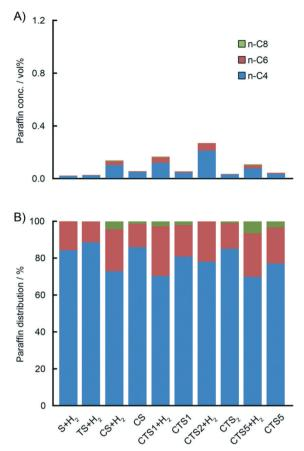
Fig. 8 GC analysis of the gas phase during ethylene polymerisation with various Phillips-type catalysts showing different gas phase concentrations (A) of the in situ produced C4 (blue), C6 (red) and C8 (green) paraffins depending on the catalyst composition. Paraffin distribution normalised to 100% (B) reveals that the titanation of the Phillips-type catalysts does not change significantly the ratio of produced oligomers.
