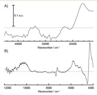
Fig. 4 Difference spectrum of the catalyst modified with TEAl and the fresh Cr/SiO<sub>2</sub> Phillips-type catalyst in the UV-vis (A) and the vis-NIR (B) region showing the reduction of some of the Cr<sup>6+</sup> species as testified by the negative  $O \rightarrow Cr^{6+}$  charge transfer bands and positive bands of the formed Cr<sup>3+</sup> and Cr<sup>2+</sup> species at approximately 16 000 and 10 000 cm<sup>-1</sup>, respectively. Zero is presented with the red line.
