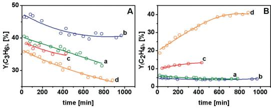
Fig. 8 Yields of  $C_3H_6$  (panel A) and  $C_2H_4$  (panel B) vs. reaction time during ODH of propane on the 2.0-Cr/DHS catalyst (T=873 K, w=200 h<sup>-1</sup>) under different reaction conditions: a)  $C_3H_8: N_2 = 15:85$  (green); b)  $C_3H_8: CO_2: N_2 = 15:30:55$  (blue); c)  $C_3H_8: O_2: N_2 = 15:3:82$  (red); d)  $C_3H_8: CO_2: N_2 = 15:3:82$  $CO_2: O_2: N_2 = 15:30:3:52$  (orange).
