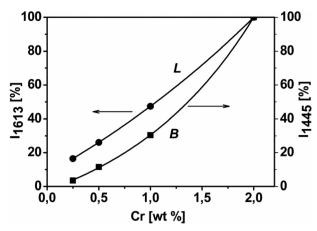
Fig. 5 Relative integrated intensity of the IR absorption bands of NH<sub>3</sub> adsorbed on Cr/DHS samples, due to Lewis (L, band at 1613 cm<sup>-1</sup>) and Brønsted (B, band at 1445 cm<sup>-1</sup>) acidity vs. chromium content. Original spectral data are shown in Fig. S5A in the ESI.†
