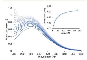
Fig. 4 UV-vis titration showing addition of aliquots of a pyridine solution to an aqueous suspension of Cu(1) nanosheets. Inset shows a plot of change in absorbance against concentration of pyridine which is fitted to calculate the binding constant for pyridine to the nanosheets ( $K_a = 30 \pm 8 \ M^{-1}$ ).
