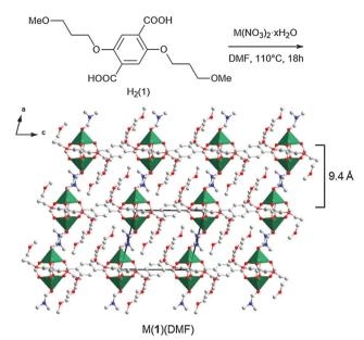
Fig. 1 Reaction scheme for the synthesis of M(1)(DMF) (with M = Cu, Zn) showing the crystal structure of Zn(1)(DMF) viewed along the b-axis highlighting the lamellar structure with an interlayer spacing of  $\sim 9.4 \text{ Å}$  $(\sim 9.6 \text{ Å for Cu}(\mathbf{1})(\text{DMF}))$ . C, N and O atoms are shown in grey, blue and red. The coordination polyhedra of the M ions are displayed in green. H atoms have been omitted for clarity.
