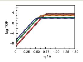
Fig. 5 Catalytic Tafel plot. Turnover frequency for the evolution of hydrogen from 1 M acetic acid in DMF catalysed by 1 (— blue), 2 (green), 3 (- orange), 4 (- red) and 5 (- brown) as a function of overpotential.
