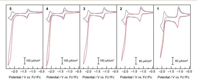
Fig. 6 Cyclic voltammograms under Ar (— blue) and  $CO_2$  (— red) at 50 mV s<sup>-1</sup> of 1 mM solutions of compounds 1–5 in DMF/H<sub>2</sub>O (95 : 5), TBAPF<sub>6</sub> 0.1 M.
