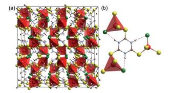
Fig. 1 Crystal structure of [CuCl(ttcH $_3$ )]. $^{13}$  (a) 2 × 2 × 2 cells. (b) Connectivity of CuClS $_3$  tetrahedral with the thioketone form of trithiocyanuric acid molecules (red: Cu, green: Cl, yellow: S, blue: N, brown: C, and white: H). Dotted lines show hydrogen bonding.
