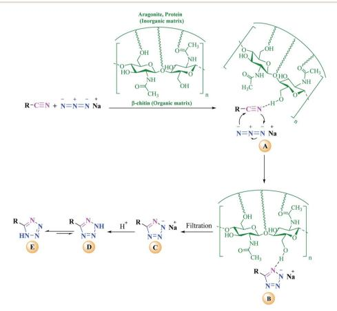
Scheme 2 Proposed mechanism for the synthesis of 5-substituted-1*H*-tetrazoles in the presence of cuttlebone.
