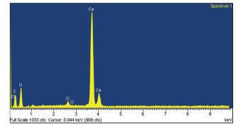
Fig. 6 EDS of finely powdered cuttlebone.
