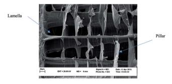
Fig. 4 SEM image of cuttlebone.
