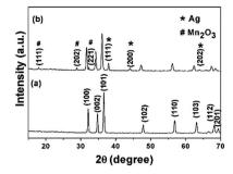
Fig. 1 XRD patterns of the synthesized (a) pure ZnO and (b) ternary  $\text{ZnO/Ag/Mn}_2\text{O}_3$  nanocomposite.
