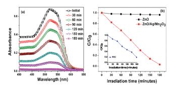
Fig. 5 (a) UV-vis absorbance spectra, and, (b) time course degradation curves of industrial textile effluents using pure ZnO and ternary ZnO/Ag/Mn $_2$ O $_3$  nanocomposite and inset shows TOC result under visible light irradiation.
