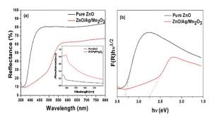
Fig. 4 (a) UV-vis diffuse reflectance spectra, and the inset shows UV-vis absorption spectra, and, (b)  $F(R)h\nu^{1/2}$  vs.  $h\nu$  plot of the pure ZnO and ternary ZnO/Ag/Mn<sub>2</sub>O<sub>3</sub> nanocomposite.
