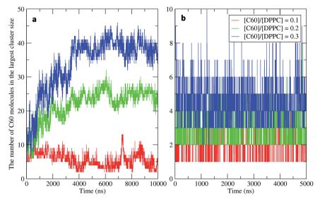
Fig. 4 Time evolution of the largest cluster size in the systems of 400 molecules per monolayer for different [ $C_{60}$ ]/[DPPC] ratios at the area per molecule of (a) 0.48 nm<sup>2</sup> and (b) 0.60 nm<sup>2</sup>.
