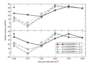
Fig. 1 Surface tension/area isotherms with different  $C_{60}$ /DPPC ratios for (a) small systems (400 molecules per monolayer) and (b) large systems (1600 molecules per monolayer). The error bars are of the size of the symbols.
