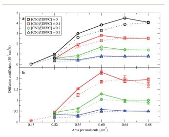
Fig. 7 Diffusion coefficients of (a) DPPC lipids and (b) fullerenes as a function of the area per molecule. The systems consisted of 400 (dot line) and 1600 (solid line) molecules per monolayer. The error bars for DPPC are of the size of the symbols. Diffusion coefficients were not calculated in simulations with an area per molecule of 0.48 nm<sup>2</sup> and [C<sub>60</sub>]/[DPPC] ratios of 0.2 and 0.3 because the monolayers collapsed.
