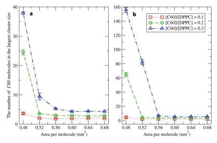
Fig. 5 The average largest cluster size as a function of the area per molecule in the systems of (a) 400 and (b) 1600 molecules per monolayer at different  $[C_{60}]/[DPPC]$  ratios.
