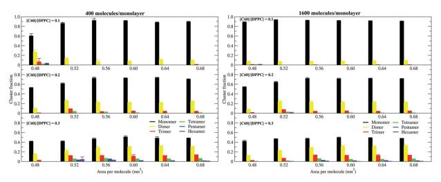
Fig. 6 Population of monomeric and aggregated fullerene as a function of the area per molecule, in systems of 400 (left panel) and 1600 (right panel) molecules per monolayer, at different [C<sub>60</sub>]/[DPPC] ratios.
