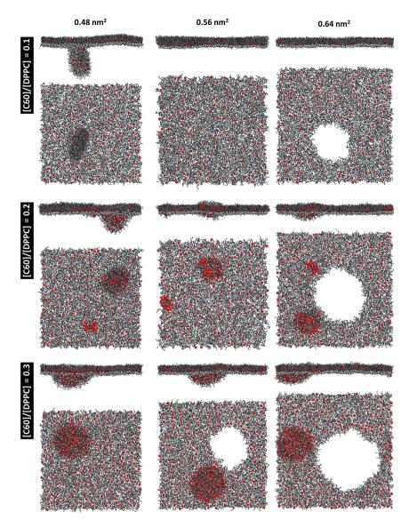
Fig. 8 The  $0.48 \text{ nm}^2$  systems were expanded to  $A=0.56 \text{ nm}^2$  and  $A=0.64 \text{ nm}^2$ , and then equilibrated for  $1 \mu s$ . The simulations consisted of 1600 molecules per monolayer with varying [C<sub>60</sub>]/[DPPC] ratios. Lipids are shown in gray and fullerenes in red. Water beads are not shown for clarity.
