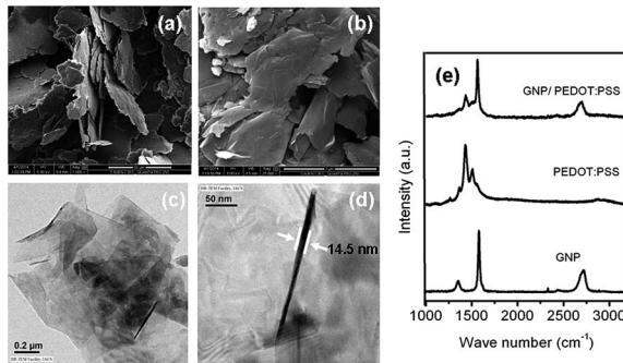
**Fig. 1** Scanning electron micrographs of the GNPs (a) and GNP/PEDOT:PSS composite (b). (c and d) Transmission electron micrographs of a GNP/PEDOT:PSS composite with 10% GNPs. (d) reveals that the thickness of the GNPs is ~15 nm. (e) Raman spectra of the GNPs, PEDOT:PSS and the GNP/PEDOT:PSS composite with 10 wt% GNPs.
