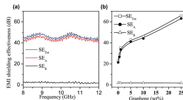
Fig. 3 (a) The comparison between  $\text{SE}_{\text{Tot}}$ ,  $\text{SE}_A$  and  $\text{SE}_R$  for the graphene/PEDOT:PSS sample with 10% graphene loading, and (b) the same for samples with different graphene loadings at 10 GHz.
