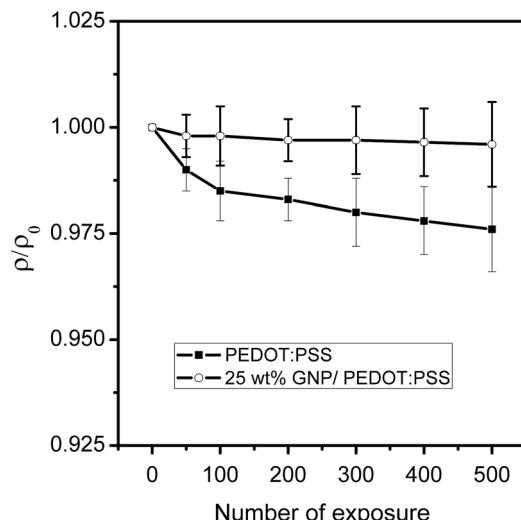
Fig. 4 Resistivity ratio vs. number of exposures for the samples with 25 wt% GNP/PEDOT:PSS and pristine PEDOT:PSS.  $\rho_0$  being the initial resistivity.
