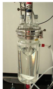
Fig. 11 \text{MgF}_2 sol stabilised by \text{Al}(\text{O}'\text{Pr})_3 after 2 days of fluorination prepared in a 10 L reactor.
