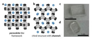
**Fig. 1** Schematics of the two structure types observed in the series  $[NH_3NH_2]B(HCOO)_3$  with  $B=Mn^{2+}$ ,  $Co^{2+}$ ,  $Zn^{2+}$  and  $Mg^{2+}$ . The structures are simplified to emphasize the perovskite-structure motif in (a) and the hexagonal channels in (b). Grey polyhedrons are  $ZnO_6$  octahedrons, black spheres formate anions and blue spheres correspond to  $[NH_3NH_2]^+$  cations. (c and d) Show crystals of **Zn-1** (c) and **Zn-2** (d), see ESI† for more crystals.
