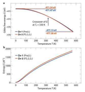
**Fig. 2** Temperature dependence of the Gibbs free energy G (a) and entropy S (b) of the compounds **Zn-1** (blue) and **Zn-2** (orange). With increasing temperature, the entropic contribution becomes more dominant which causes the crossover of G at  $T_{\rm c}$  = 330 K. The higher vibrational entropy of the channel structure is caused by a lower density and weaker hydrogen bonding pattern.
