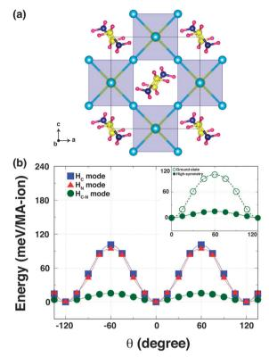
Fig. 3 (a) A high-symmetry structure characterised by the removal of octahedral tilting in o-MAPbl $_3$ . (b) The K–S energies plotted as a function of the torsion angle  $\theta$  for three rotational modes in the high-symmetry structure. Inset compares the energy barriers for the H $_{C-N}$  mode in the high-symmetry structure and the ground-state structure with octahedral tilting.
