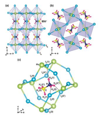
Fig. 1 (a) Optimized crystal structure of o-MAPbI $_3$ , viewed in the a-b and, (b) a-c planes. PbI $_6$  octahedra are highlighted in purple. (c) Local cage structure of o-MAPbI $_3$  is characterized by hydrogen-bonding between the three H atoms in the NH $_3$  group and one axial I [I $_4$ (1)] atom and two equatorial I [I $_6$ (2) and I $_6$ (2')] atoms. Hydrogen-bonding interactions are indicated by dotted lines.
