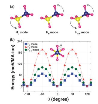
Fig. 2 (a) Schematic view of three MA rotational modes (see text). (b) The computed Kohn-Sham (K-S) energies as a function of the torsion angle  $\theta$ for the three rotational modes and a staggered conformation (inset) with the torsion angle  $\theta = 0^{\circ}$ .
