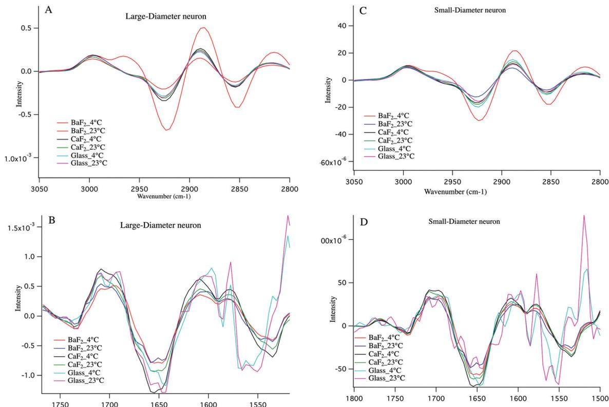
**Fig. 6** Second derivative average spectra for large diameter (A, B) and small diameter (C, D) DRG neurons in protein region (B, D) and lipid region (A, C) for BaF<sub>2</sub>\_4 °C, BaF<sub>2</sub>\_23 °C, CaF<sub>2</sub>\_4 °C, CaF<sub>2</sub>\_23 °C, glass\_4° and glass\_23 °C are shown. It clearly shows that the neurons maintained at 4 °C and plated on BaF<sub>2</sub> window has higher intensity in the spectral component associated with lipid, compared to the other conditions.
