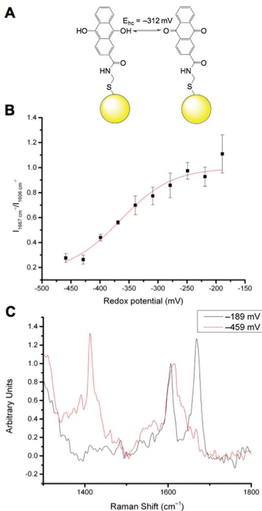
**Fig. 2** AQ-NP nanosensor. (A): Equilibrium between oxidised and reduced AQ attached to a gold NP (yellow sphere, not to scale). (B): Calibration curve for AQ-NP nanosensors ( $R^2 = 0.96855$ ). (C): Representative spectra of fully oxidised ( $-189$  mV) and fully reduced ( $-459$  mV) AQ-NPs.
