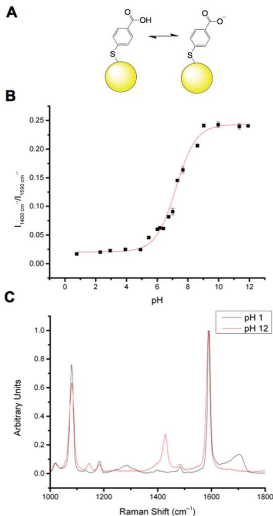
**Fig. 1** MBA-NP nanosensor. (A): Equilibrium between protonated and deprotonated MBA attached to a gold NP (yellow sphere, not to scale). (B): Calibration curve for MBA-NP nanosensors ( $R^2 = 0.98687$ ). (C): Representative spectra of fully protonated (pH 1) and fully deprotonated (pH 12) MBA-NPs.
