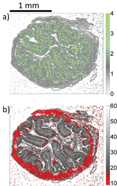
**Fig. 5** Microscopic images resulting from the analysis of infrared data of the training set. (a) Represents the ratio of absorbances at  $1076\text{ cm}^{-1}$  and  $1181\text{ cm}^{-1}$ . (b) Represents the integral absorbance over the  $1027\text{ cm}^{-1}$ – $1087\text{ cm}^{-1}$  spectral range (see also in Table 1).
