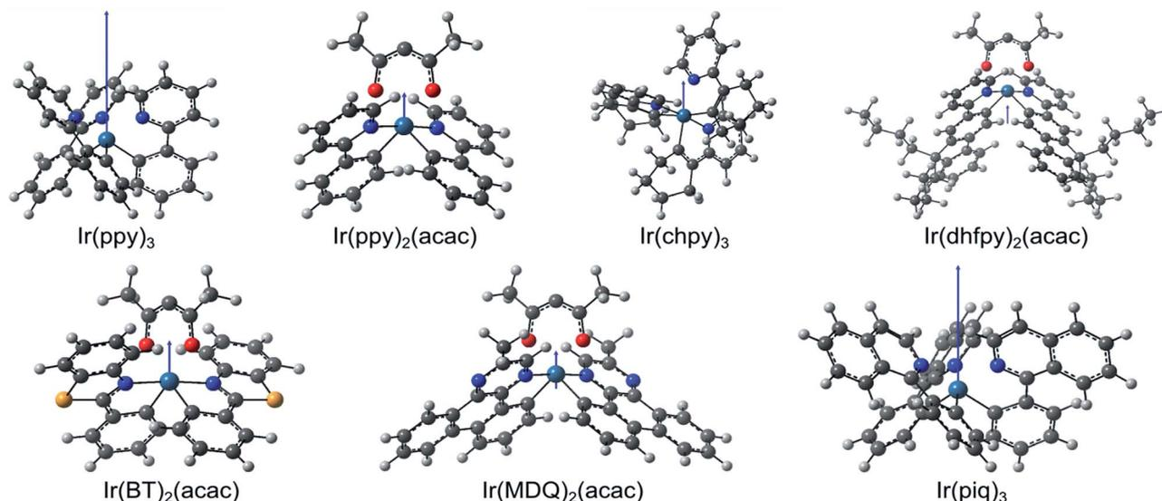
Fig. 3 DFT optimized molecular structure, calculated relative magnitude and orientation of permanent dipole moment  $\mu$  (blue arrows) for all phosphorescent emitter molecules investigated here. All dipole moments originate at the center of charge.
