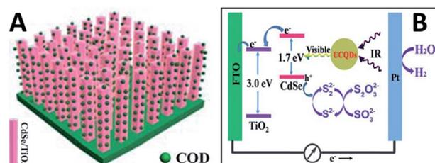
Fig. 29 (A) A schematic diagram showing the CQD/CdSe/TiO<sub>2</sub> NR photoanode. (B) A schematic diagram to illustrate how up-conversion of the carbon quantum dots (UCQDs) served as spectral converters for the CdSe/TiO<sub>2</sub> NR photoanode. Adapted with permission.<sup>126</sup> Copyright 2013, Royal Society of Chemistry.
