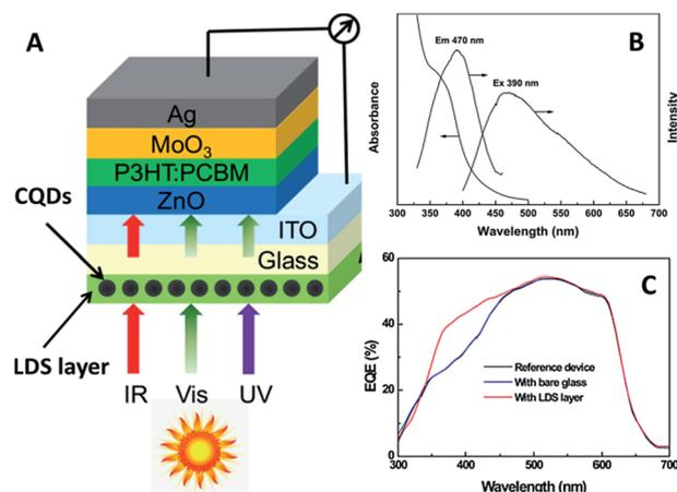
Fig. 26 (A) Schematic architecture of the BHJ solar cell with LDS layer. (B) UV-vis absorption and PL spectra of the CQDs filled polysiloxane composite ( $\sim 20 \mu\text{m}$  thick) coated on glass. (C) Wavelength dependences of external quantum efficiency of the P3HT:PCBM-based solar cell with and without the LDS layer. Adapted with permission.<sup>71</sup> Copyright 2014, Elsevier.
