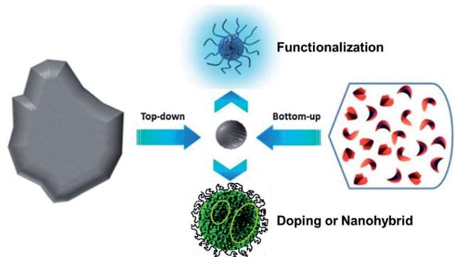
Fig. 2 Schematic illustration of CQDs preparation *via* “top-down” and “bottom-up” approaches, and modification including functionalization, doping and nanohybrids. Adapted with permission.<sup>8</sup> Copyright 2013, Royal Society of Chemistry.
