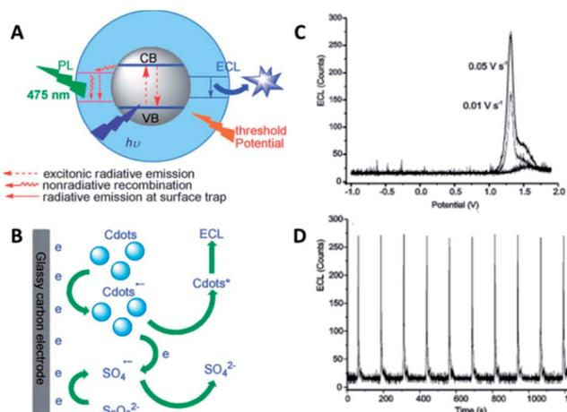
Fig. 15 (A) Schematic illustration of the PL and ECL emissions of CQDs. (B) The mechanism of ECL in the o-CQDs/ $K_2S_2O_8$  system. (C) ECL profiles of o-CQDs at a scan rate of 0.01 and 0.05  $V s^{-1}$ . (D) The reproducibility of ECL in a continuous scan mode. Adapted with permission.<sup>78</sup> Copyright 2013, Wiley-VCH.
