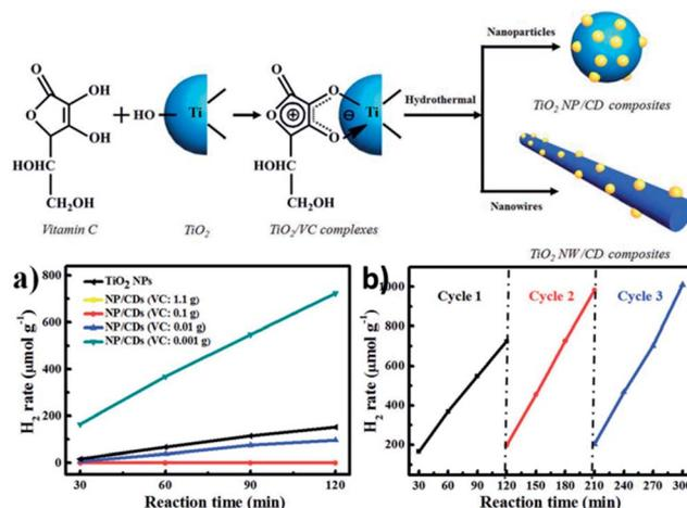
Fig. 11 (Up) Schematic illustration of the *in situ* hydrothermal synthesis of TiO<sub>2</sub>/CQD nanohybrids. (Down) (a) Time course of H<sub>2</sub> production from TiO<sub>2</sub> NPs and NP/CQDs composites synthesized at different VC amounts: 1.1, 0.1, 0.01 and 0.001 g. (b) A typical time course of H<sub>2</sub> production from NP/CQDs composites for 3 cycles. Adapted with permission.<sup>69</sup> Copyright 2014, Royal Society of Chemistry.
