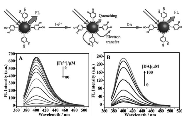
Fig. 30 (Up) Schematic representation of fluorescent CQDs for the detection of Fe<sup>3+</sup> ions and dopamine. (A) Representative fluorescence emission spectra of CQDs in the presence of increasing Fe<sup>3+</sup> concentration (0–700 μM) in a HEPES buffer (10 mM) at pH 7.0. (B) Fluorescence emission spectra of CQDs containing Fe<sup>3+</sup> (600 μM) with increase in DA concentration (0–100 μM). Adapted with permission.<sup>61</sup> Copyright 2013, Wiley-VCH.
