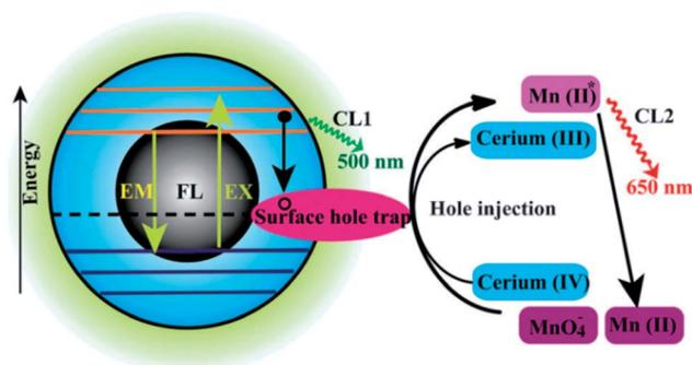
Fig. 14 Schematic illustration of the FL and CL mechanisms in the CQDs– $\text{KMnO}_4$  and CQDs–cerium(IV) systems. CL1 and CL2 represent two CL routes in the system. Adapted with permission.<sup>73</sup> Copyright 2012, Royal Society of Chemistry.
