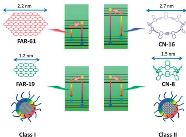
Fig. 19 Schematic illustration of the PL mechanism of Class I and Class II CQDs. Adapted with permission.<sup>8</sup> Copyright 2013, Royal Society of Chemistry.
