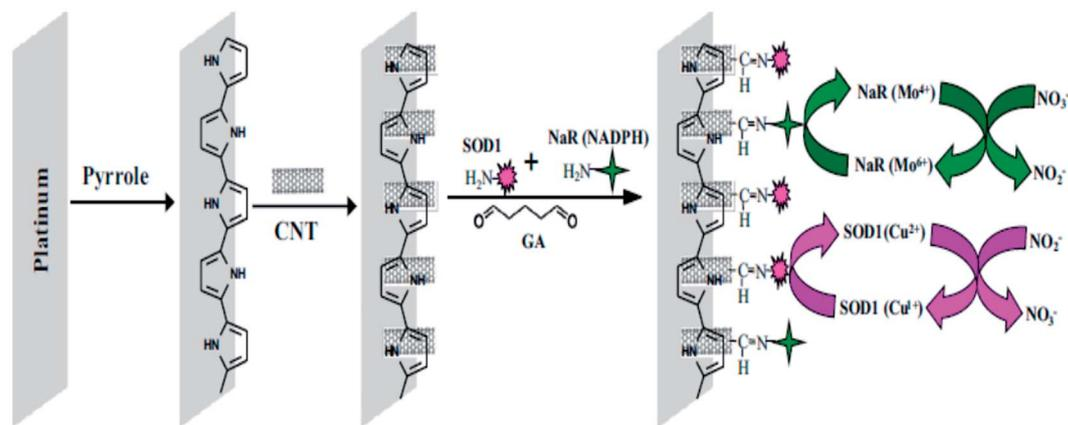
Fig. 6 Construction of a NaR-SOD1-CNT-PPy-Pt electrode and reactions involved during the simultaneous determination of NO<sub>2</sub><sup>-</sup> and NO<sub>3</sub><sup>-</sup>. Reproduced with permission from ref. 126 © 2014 Elsevier.
