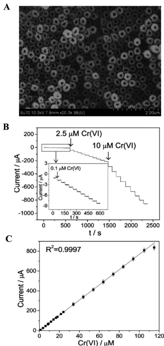
Fig. 5 (A) SEM image of the Au NPs decorated TiO<sub>2</sub>NT electrode. (B) Amperometric responses at the Au nanoparticle decorated TiO<sub>2</sub>NT electrode for the successive addition of Cr(VI) with a polarized potential of  $0.28 \text{ V}$  in  $0.1 \text{ M HCl}$ . (C) Calibration plot of corresponding amperometric response. Reproduced with permission from ref. 70 © 2014 Royal Society of Chemistry.
