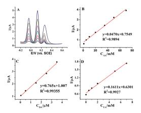
Fig. 5 (A) DPV profiles at AuNPs@MoS<sub>2</sub>/GCE in 0.1 M PB solution (pH 7.0) containing different concentrations of AA, DA and UA. From bottom to up the concentrations from 1 mM to 70 mM for AA, 0.01  $\mu$ M to 7  $\mu$ M for DA and 0.01 mM to 12 mM for UA, respectively. (B–D) The plots of the oxidative peak currents *versus* the concentrations of AA, DA and UA.
