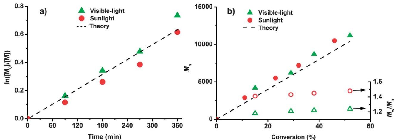
Fig. 5 Visible light- or sunlight-induced ATRP of methyl methacrylate with low copper catalyst loading ( $[MMA]_0/[EtBP]_0/[Cu^{II}Br_2]_0/[PMDETA]_0/[Mn_2(CO)_{10}]_0 = 200/1/0.01/0.01/0.05$ ): (a) kinetic plot and (b) molecular weights and distributions of the resulting polymers as a function of degree of conversion.
