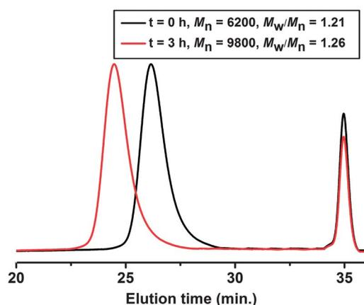
Fig. 7 GPC traces of the PMMA-Br macroinitiator before and after chain extension via visible light-induced ATRP using  $Mn_2(CO)_{10}$ . Experimental conditions:  $[MMA]_0/[PMMA-Br]_0/[Cu^{II}Br_2]_0/[PMDETA]_0/[Mn_2(CO)_{10}]_0 = 200/1/0.01/0.01/0.05$  ratio.
