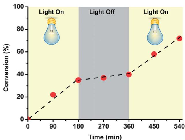
Fig. 6 Effect of visible light during the polymerization of MMA at room temperature:  $[MMA]_0/[EtBP]_0/[Cu^{II}Br_2]_0/[PMDETA]_0/[Mn_2(CO)_{10}]_0 = 200/1/0.2/0.2/0.05$ .
