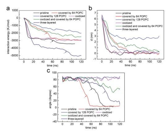
Fig. 3 The evolution of (a) interaction energy, (b) distance and (c) angle between lipid bilayer and a nanosheet of graphene that is pristine (black), coated with 64 (red) and 128 (blue) POPC lipids, oxidized (magenta), three-layered (dark blue), oxidized and coated by 64 POPC lipids (green). For comparison purposes, the profiles for pristine graphene (black) have been shifted by 73.5 ns leftwards.
