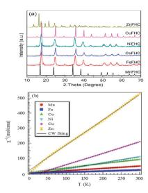
**Fig. 2** (a) XRD patterns of Prussian blue compounds. (b)  $\chi_{\rm m}^{-1}$ -T plot of Prussian blue compounds.
