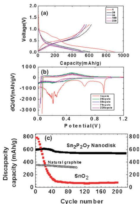
**Fig. 2** (a) Voltage profiles of the quenched nanodisks in a coin-type half cell between 0 and 1.2 V at 0.5 C rate ( $= 350 \text{ mA g}^{-1}$ ) after 1, 20, 50, 100, 220 cycles. (b) Differential curves of (a). (c) Discharge capacity (after lithium removal) vs. cycle number in nanodisk. References are natural graphite and  $\text{SnO}_2$  nanoparticles.
