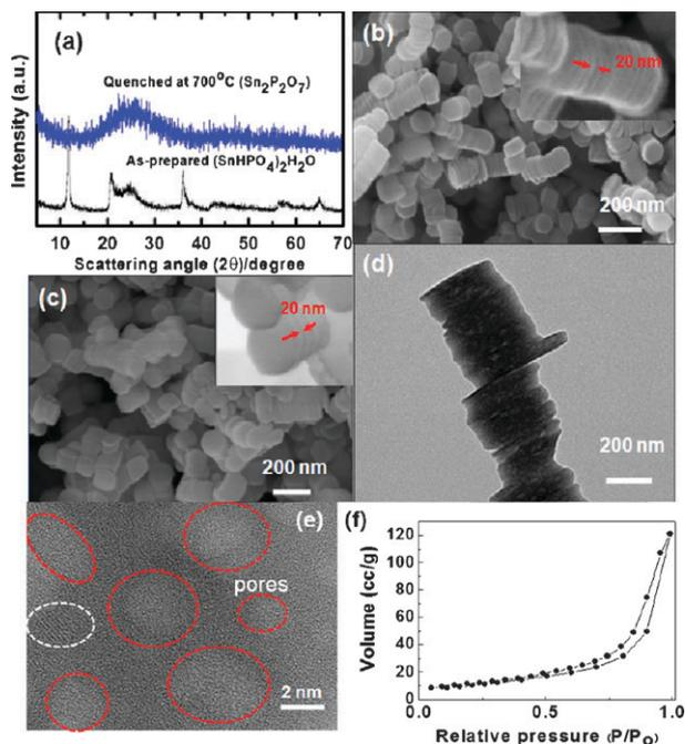
**Fig. 1** (a) XRD patterns of as-prepared and quenched nanodisks at 700 °C. (b, c) SEM images of as-prepared and quenched nanodisks at 700 °C (insets: expanded images of b and c). (d) TEM image of the quenched nanodisk where white spots indicate the mesopores. (e) Expanded image of (d) where red circles indicate the mesopores and the white circle indicates a possible crystalline domain. (f)  $\text{N}_2$  isotherm of the quenched sample.
