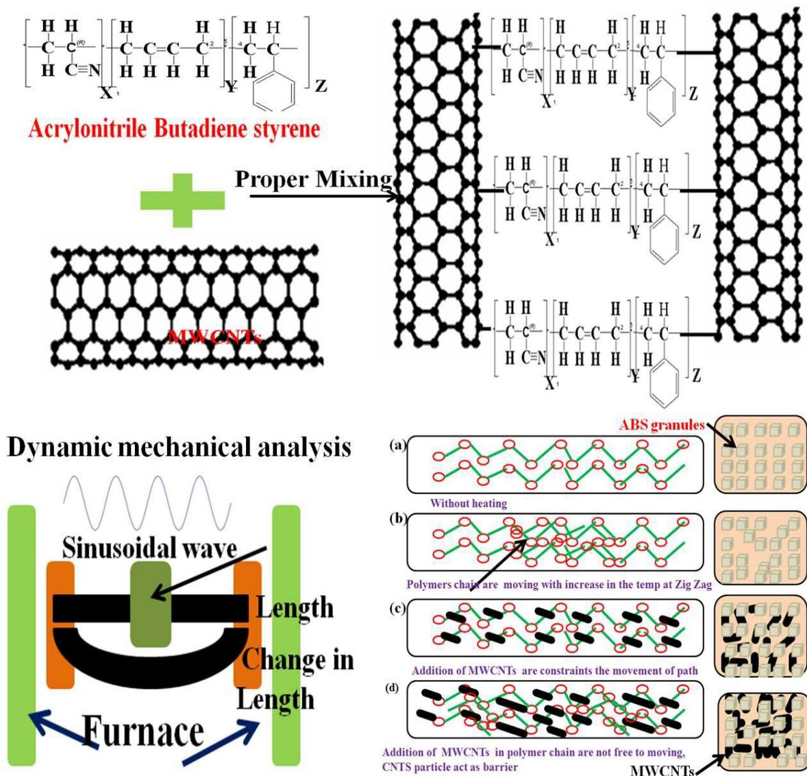
**Fig. 1** Schematic representation of mixing of MWCNTs and ABS, interaction of the MWCNTs and ABS and DMTA studies with variation of the temperature.
