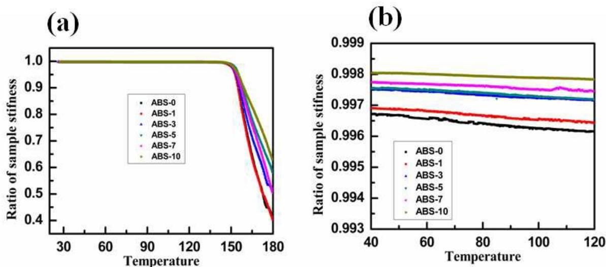
**Fig.11 (a) Ratio of the sample stiffness vs. temperature plot for different wt % of MWCNTs/ABS composites (b) at the lower range of the temperature scale (zoom**
