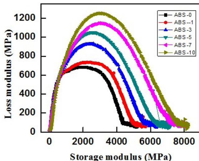
**Fig. 12 Cole-Cole plots of pure ABS and MWCNTs/ABS composites**
