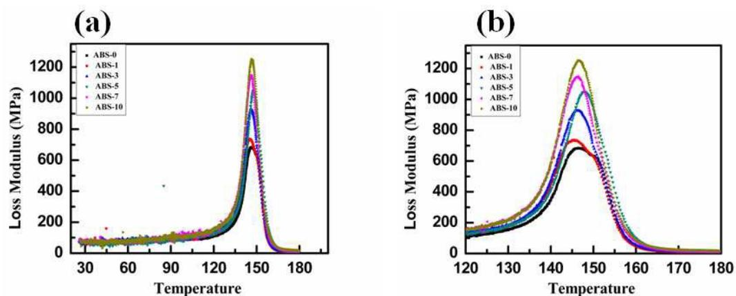
**Fig. 7** Variation of (a) loss modulus with temperature (b) zoomed plot between 120 to 180°C for different wt % of MWCNTs/ABS composites
