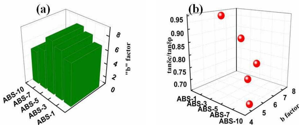
**Fig. 10.** Variation of (a) matrix interphase factor b and (b) 3D diagram for damping behaviour and b-factor for different wt % of MWCNTs/ABS composites
