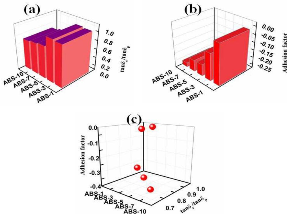
**Fig. 9** Variation of (a) Ratio of the damping factor of the composite and polymer (b) adhesion factor versus wt.% of MWCNTs and (c) 3D diagram of adhesion factor and Ratio of the damping factor of the composite and polymer for different wt % of MWCNTs/ABS composites
