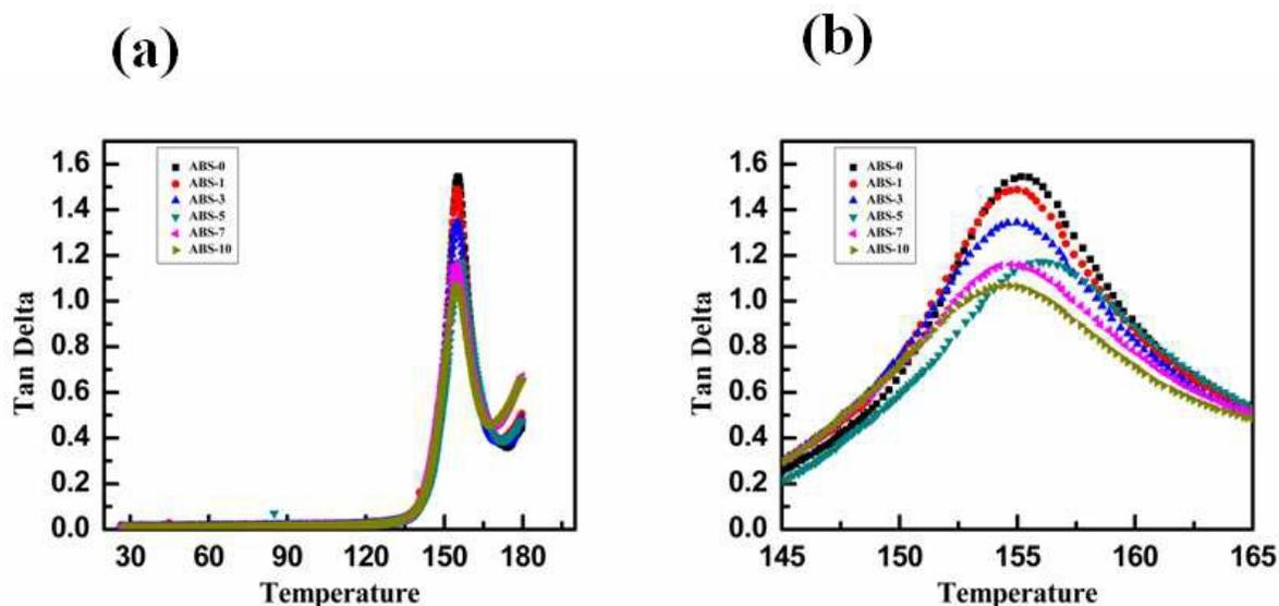
**Fig. 8** Variation of (a) Tan delta with temperature plot (b) zoomed part between 145 - 165°C for different wt % of MWCNTs/ABS composites
