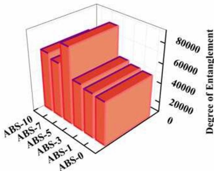
**Fig 5. Variation in degree of the entanglement factor with wt. % of MWCNTs in the ABS matrix at 150°C**
