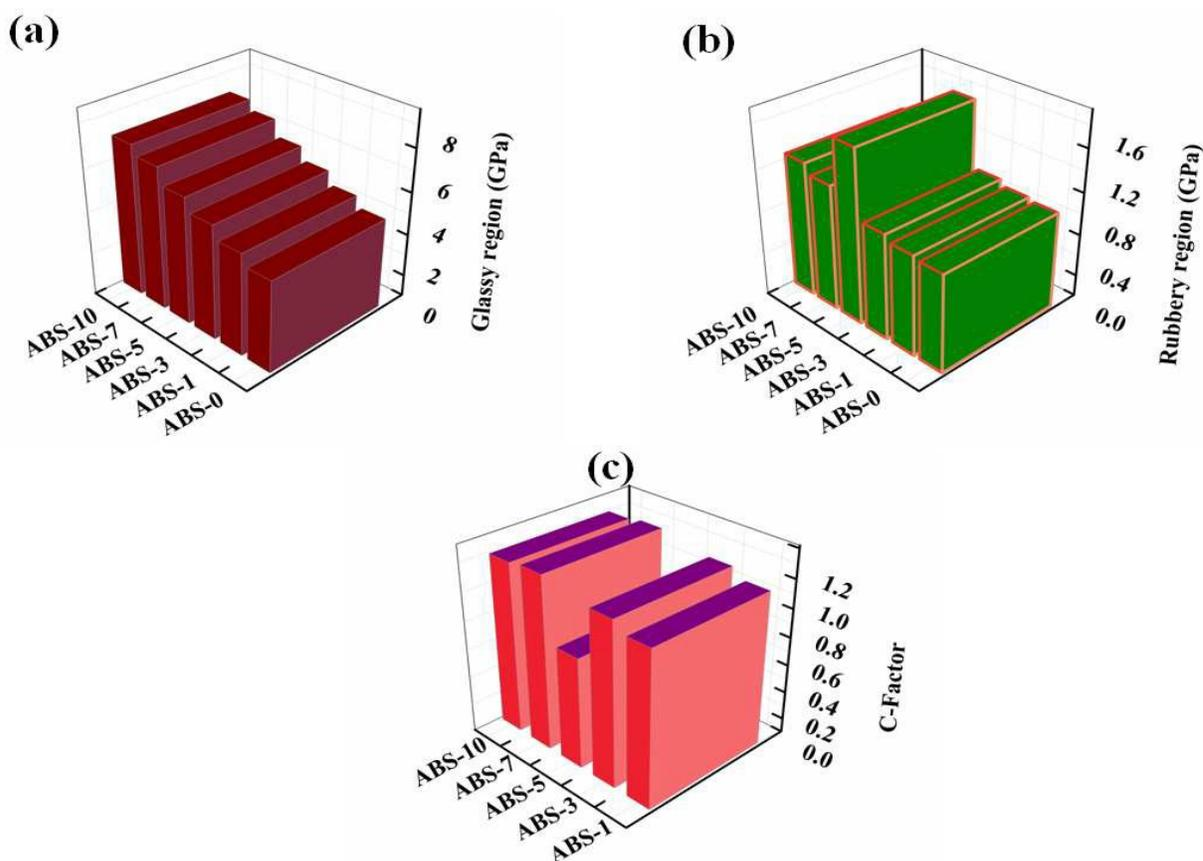
**Fig 4. Variation in (a) storage modulus in the glassy region (130°C) (b) storage modulus in the rubbery region (150°C) and (c) Coefficient of “C” factor with the weight percentage of MWCNTs in ABS matrix**
