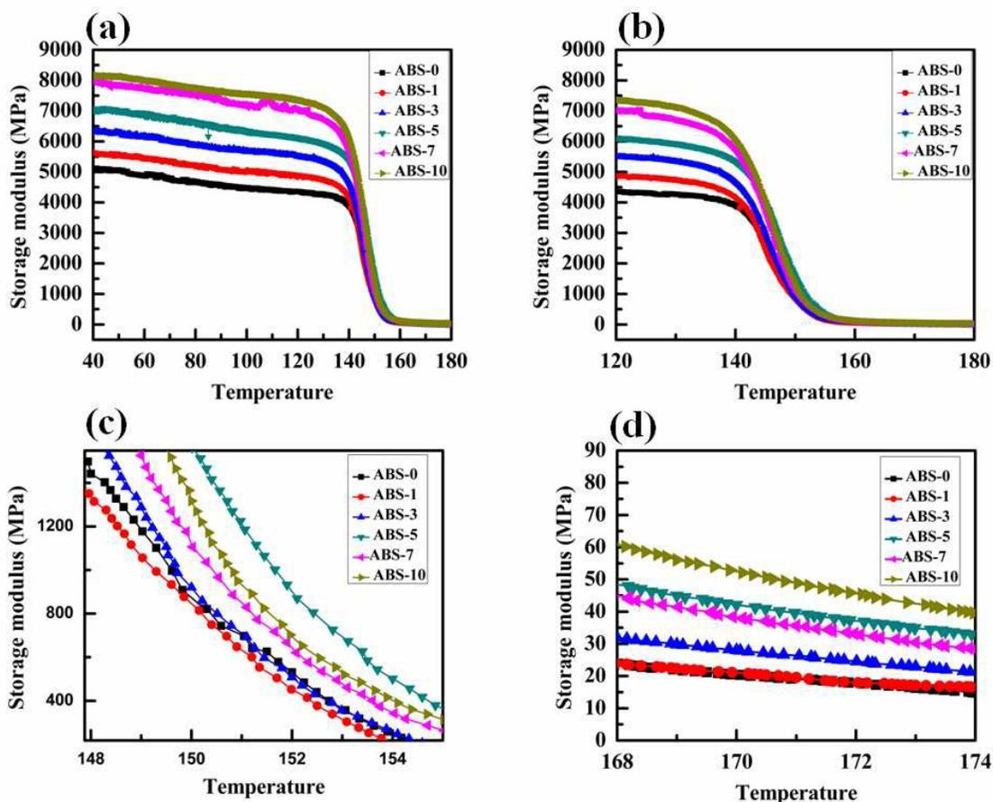
**Fig 3** Variation of (a) Storage modulus with temperature, zoomed plot (b) between 120 to 180°C , (c) between 148 to 155°C, (d) between 168 to 174°C for different wt % of MWCNTs/ABS composites
