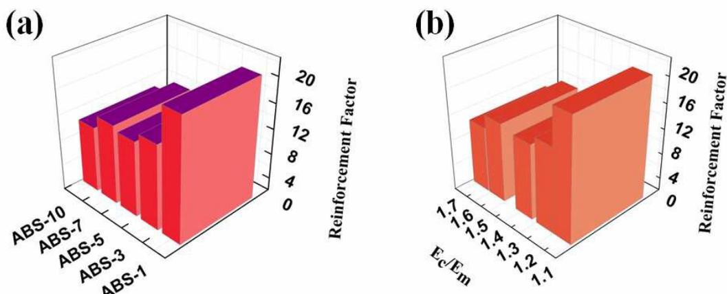
**Fig. 6 (a) Variation of Reinforcement factor with wt. % of MWCNTs in the ABS matrix (b) ratio of storage modulus of polymer composites and pure polymer with reinforcement factor**
