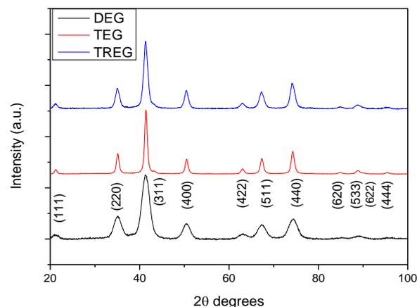
Figure 5. XRD pattern of IONPs synthesized in different polyol solvents (DEG, TREG and TEG). Peaks have been indexed according to the reference pattern for magnetite (pdf ref 01-088-0315). Diffraction patterns have been normalised and offset along the y-axis for better comparison
