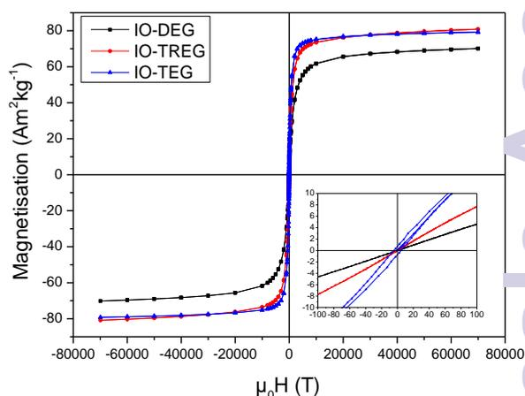
Figure 2 Magnetisation curves of IONPs obtained with different polyols (DEG, TREG and TEG)
