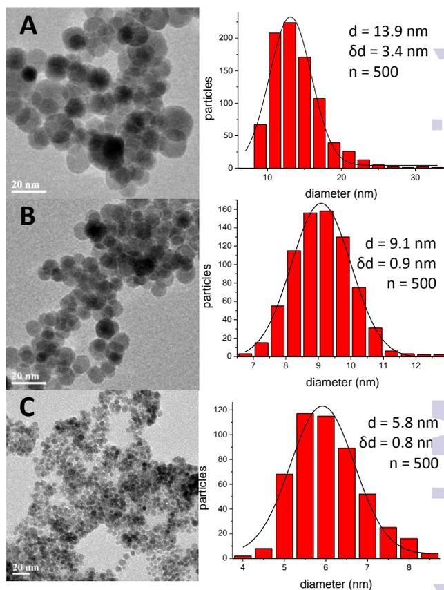
Figure 1 TEM images and particle size distributions of iron oxide nanoparticles synthesized using different polyols A) TEG, B) TREG and C) DEG. Size distributions were fitted with a normal function (solid line),  $d$  = mean diameter,  $\delta d$  = standard deviation and  $n$  = number of particles counted.
