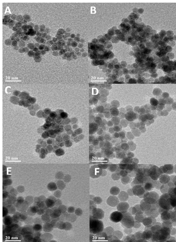
Figure 4 TEM images of iron oxide nanoparticles synthesized using different reaction times in tri(ethylene glycol): A) 1 h, B) 2 h, C) 4 h, D) 8 h, E) 12 h, and F) 24 h.
