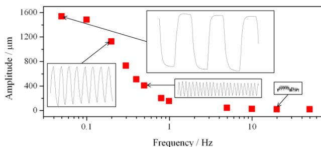
**Fig. 9.** Amplitude of the bilayer strip oscillation as a function of frequency at constant temperature and ac current ( $T = 20$  °C,  $I_{max} = 300$  mA). Inserts: tip position of the cantilever as a function of time at selected frequencies.
