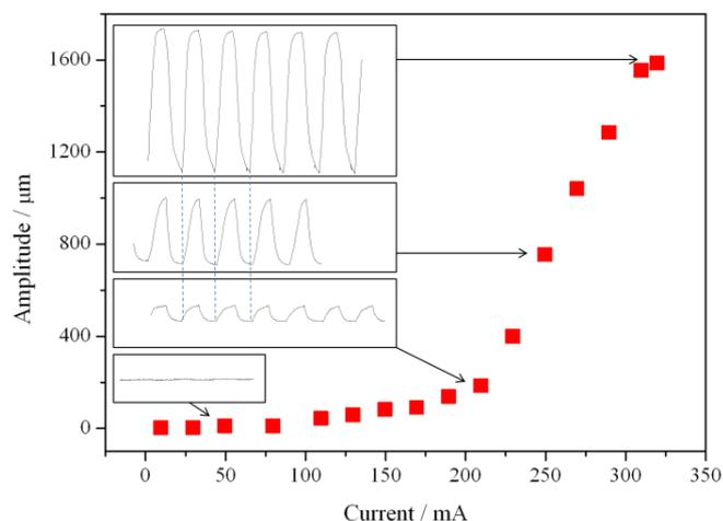
**Fig. 7.** Amplitude of oscillation of the bilayer cantilever as a function of the applied current  $I_{\text{max}}$  at constant temperature and frequency ( $T = 20 \text{ }^\circ\text{C}$ ,  $f = 0.1 \text{ Hz}$ ). Inserts: tip position of the cantilever as a function of time for a few selected values of  $I_{\text{max}}$ .
