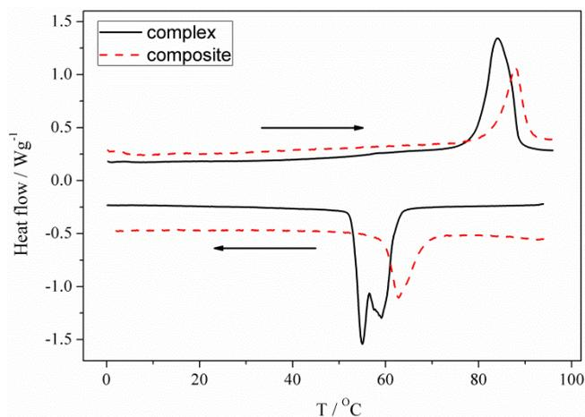
**Fig. 3.** DSC curves of the pure  $[\text{Fe}(\text{trz})(\text{H-trz})_2](\text{BF}_4)$  complex and the PMMA/ $[\text{Fe}(\text{trz})(\text{H-trz})_2](\text{BF}_4)$  (50 %) composite material acquired at heating/cooling rates of 10 °C/min.
