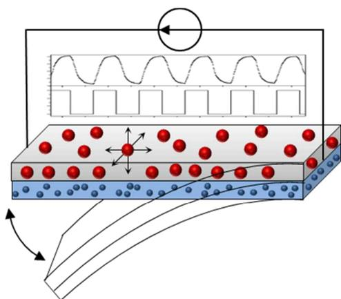
A composite bilayer actuator device which uses spin crossover to convert electrical energy into motion *via* Joule heating is described.
