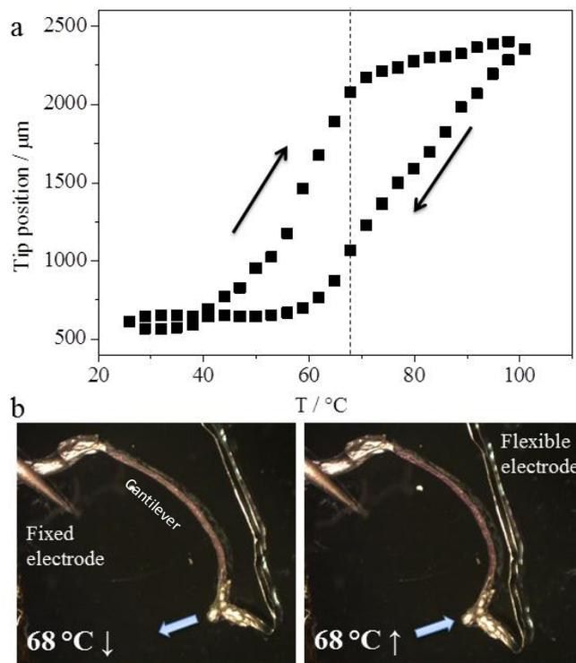
**Fig. 5.** Thermal actuation of a bimorph cantilever. (a) Tip position of the cantilever as a function of temperature. Heating and cooling modes are indicated by arrows. (b) Photographs (8.6 mm × 7.6 mm) of the cantilever at 68 °C in the cooling and heating modes demonstrate a shape memory effect, which occurs due to the thermal hysteresis of the spin transition. The color change associated with the spin transition is also observed (see also Supplemental Movie SM1).
