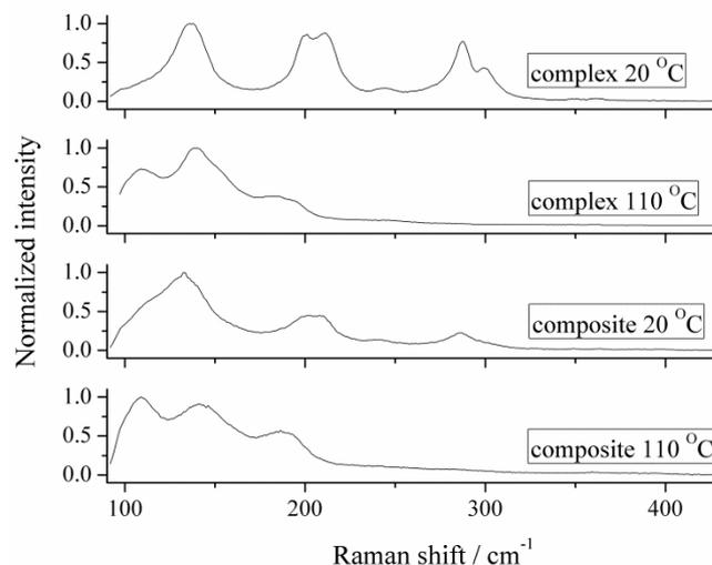
**Fig. 2.** Variable-temperature Raman spectra of the  $[\text{Fe}(\text{trz})(\text{H-trz})_2](\text{BF}_4)$  complex and the PMMA/ $[\text{Fe}(\text{trz})(\text{H-trz})_2](\text{BF}_4)$  (50 %) composite material.
