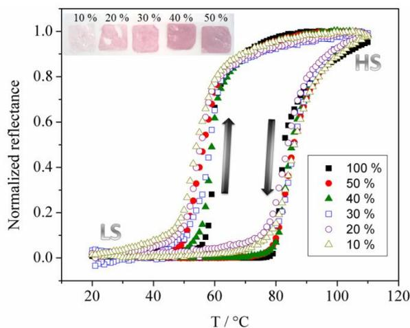
**Fig. 1.** Temperature dependence of the optical reflectance ( $\lambda = 550$  nm) of  $[\text{Fe}(\text{trz})(\text{H-trz})_2](\text{BF}_4)$  (100 %) and of the composite materials PMMA/ $[\text{Fe}(\text{trz})(\text{H-trz})_2](\text{BF}_4)$  with different loadings (10 - 50 %) of the active complex. Heating and cooling modes are indicated by arrows. The inset shows the photographs of the composite films.
