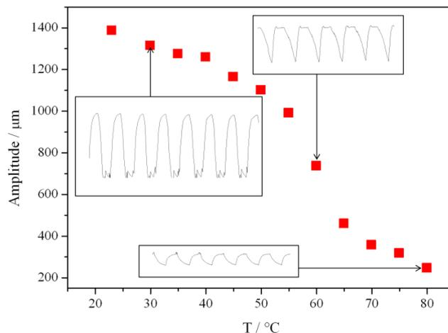
**Fig. 8.** Amplitude of the bilayer cantilever oscillation at different temperatures. The ac current and frequency were fixed ( $I_{max} = 300$  mA,  $f = 0.1$  Hz). Inserts: tip position of the cantilever as a function of time at selected temperatures.
