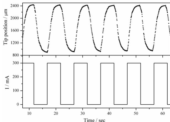
**Fig. 6.** Electric current induced actuation of a bimorph cantilever. Tip position of the cantilever as a function of time (upper panel) and the corresponding applied current signal (bottom panel). The frequency of the alternative current is 0.1 Hz,  $I_{\text{max}} = 300 \text{ mA}$ ,  $T = 20 \text{ }^\circ\text{C}$ .
