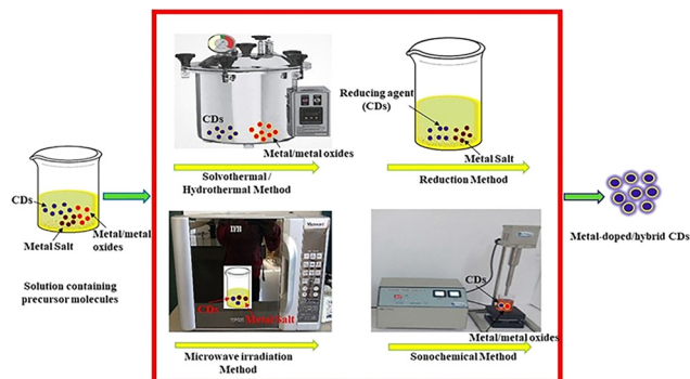
Fig. 6 Schematic representation of various methods used for synthesizing the metal-doped and hybrid CDs. Reproduced with permission. 79 Copyright 2025, Elsevier.
