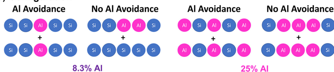
Fig. 2 Model construction outlining the three general variables. (1) Composition – stoichiometry varying with increasing Al amount. (2) Order/disorder – the topology of the model varying between the classical layered approach for C–S–H seen in literature against the “Disordered” model which represents a more homogenous blend of phases. Pore vs. hydrated pore (3) Al avoidance, resolving the influence of (non-)neighbouring Al atoms.
