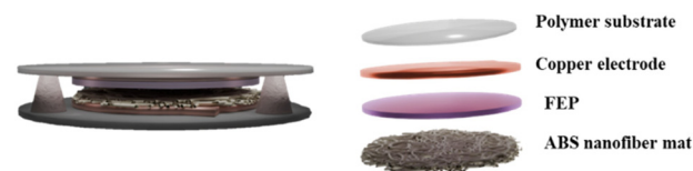
Fig. 2 Schematic representation of the ABS-based TENG.
