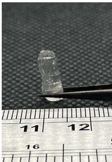
Fig. 7 PG4–Norb (1 : 1) in a large scaffold produced via photo-polymerization.
