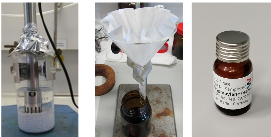
Fig. 1 Fragmentation of PP pellets with UltraTurrax (left), filtration of fragmented PP for fractionation (centre) and the final bottled PP suspension (right). 21
