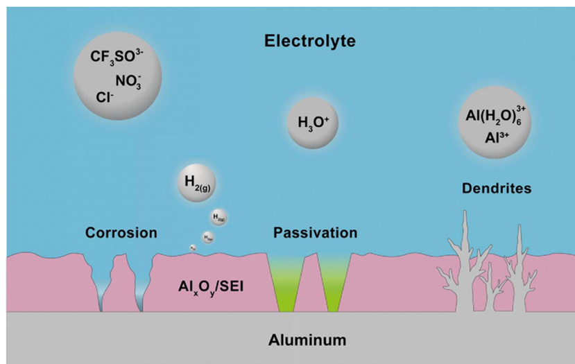
Fig. 1 Obstacles at the aluminum and electrolyte interface: illustrated explanation of possible phenomena and chemical species is shown assuming under water based electrolytes with acidic condition.
