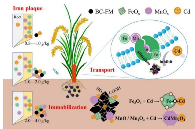
Fig. 2 Schematic diagram illustrating the passivation mechanism of Fe-Mn-based soil passivators for Cd. 65
