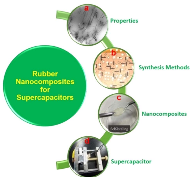
Fig. 1 Outline of the review. (a) TEM image corresponds to CNTs (10 wt%) in NR. Reproduced with permission from ref. 45 Copyright (2006) Elsevier Inc. (b) Schematic of the rGO/silica/NR composite prepared via a wet compounding procedure. Reproduced with permission from ref. 46 Copyright (2020) MDPI. (c) Digital image of the sample of S48 hydrogel. Reproduced with permission from ref. 47 Copyright (2023) Elsevier Inc. (d) Digital image of the supercapacitor during the stretching experiment. Reproduced with permission from ref. 61 Copyright (2018) MDPI.
